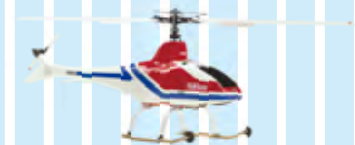
1987 Contributed to labor-saving and increased efficiency in agricultural operations R-50 (L09) industrial-use unmanned helicopter
