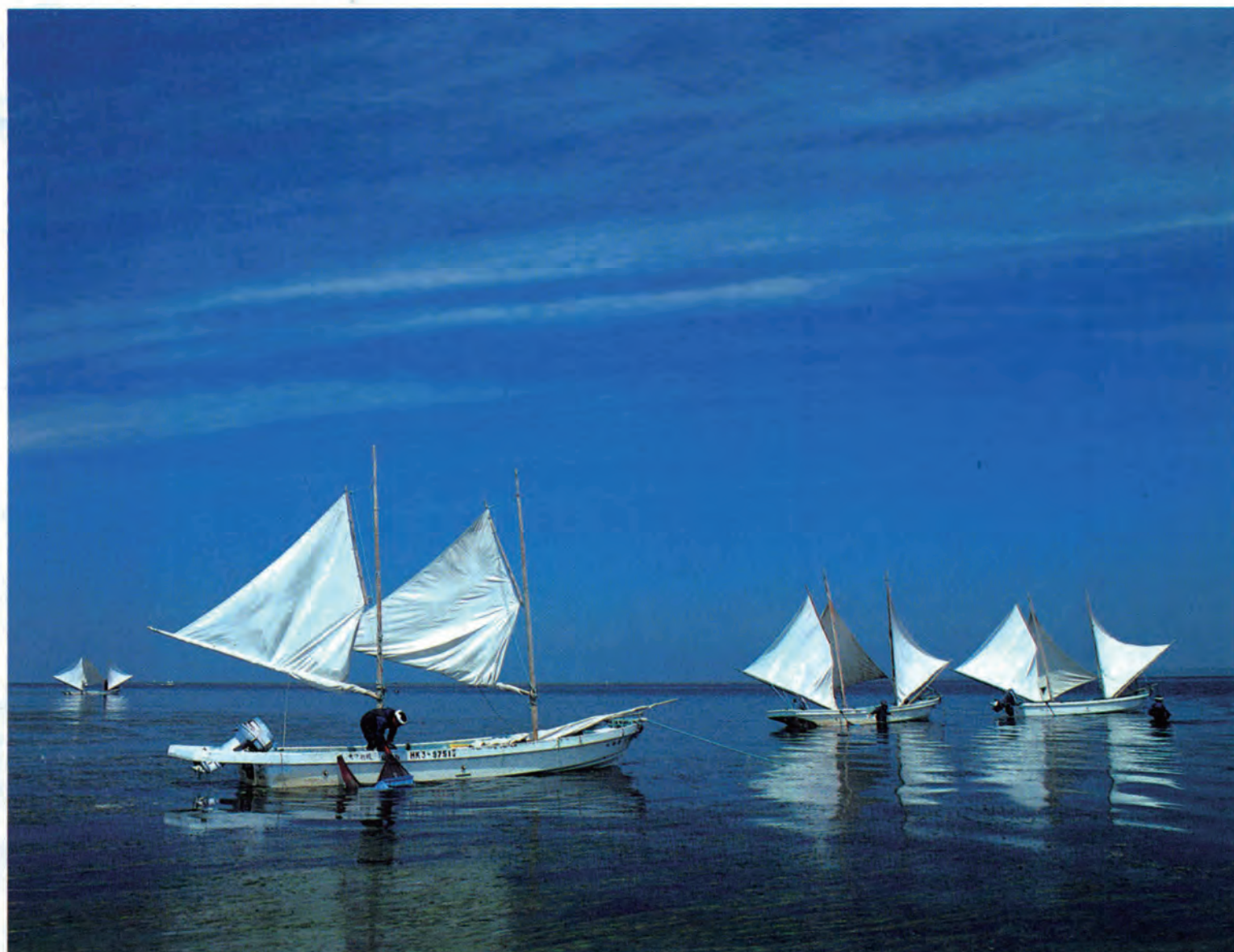
Shrimp "utase" net fishery in Notsuke Bay, Hokkaido. "Amamo" ( Zostera marina ) seaweed grows densely in areas of the bay at a depth of 2 to 5 meters. These areas are a prime habitat for northern shrimp. In utase net fishery the outboard motor is tilted up to prevent seaweed from fouling the propeller and the boat driven by a sail as the net is pulled. Notsuke Bay was first developed as a fishing ground after fishermen settled here in early 1870s. The Amamo beds are a feeding ground for shrimps and other fish fry. In order to preserve fishery resources, shrimp fishery is performed only from sail-driven boats even today, with motors used only in traveling to and from the fishing grounds. For local fishermen, utase fishery boats at work have become a symbol of resource conservation (related article on pages 4 and 5).
