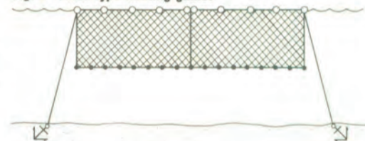
Fig. 3 Fixed-type bottom gillnet
