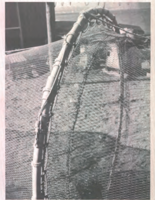
The way a funnel is attached to the bag net.
